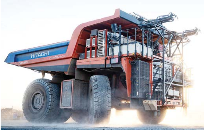
The technology, deployed at Kansanshi and Sentinel mines, uses overhead powerlines to power haul trucks on pit ramps, reducing diesel consumption by up to 90% on fully loaded up-ramps.
